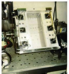
Several of our customers have contracted with us for tunrkey packages. They purchase a machine tool and send it to our facility; we design and build a fixture, program and add relays to operate the clamping mechanisms. We run samples for customer approval before it is shipped to their facility.
