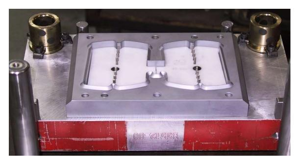
Polyuerethane trim die made from Hardened S-7 details, aluminum die set, Dayton die buttons and punches. Tolerances of .0003-.0005/ side clearance, coated with Armoloy XADC diamond impregnated coating .
