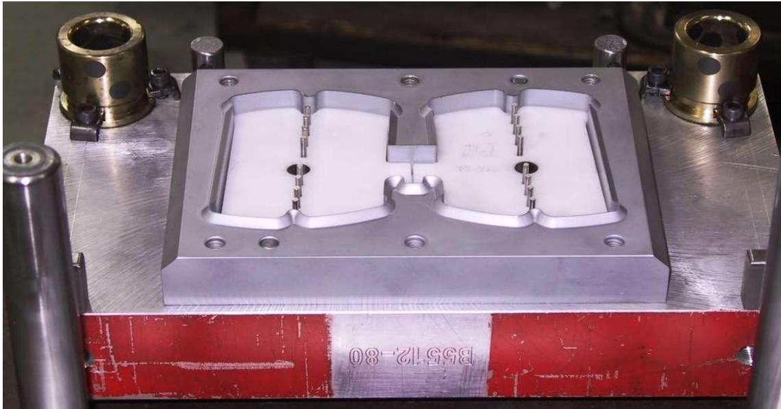
Polyurethane trim die made from Hardened S-7 details, aluminum die set, Dayton die buttons and punches. Tolerances of .0003-.0005/ side clearance, coated with Armoloy XADC diamond impregnated coating .
